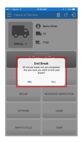
It is important to remember that in ELD mode, when the truck goes over 5MPH that the ELD will automatically move the truck into a driving status. This will occur even if you are in your 30 minute break countdown. If this happens, your 30 minute break will cancel and you will be forced to re-start the 30 minute consecutive break period again.
